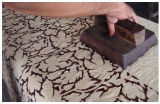
From the out line design printing, next set of Wooden Block is used with another Natural colour Dye for 2<sup>nd</sup> colour.
