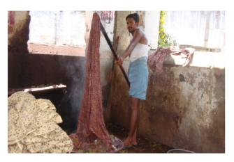
One could see that the Fabric is soaked in the Boiling water with Jagi leaves and Algrin for a while that facilitate colour fixation.
