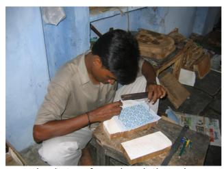
Particular design of Wooden Blocks in three printing stages, meant to be used one after the other for a 3 colour combination of block printed fabric.
