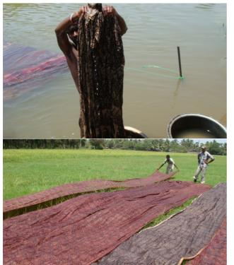
After washing the fabric, it is given treatment for colour fixing with Alumn mixed water.
